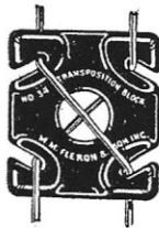
Complete glazing is an important feature of the Fleron-Wallace Block. It eliminates absorption of moisture and reduces the accumulation of soot and dirt. Only F-W Blocks have this important feature. This is the original Block adapted by Don C. Wallace on his now famous Doublet Antenna System, specifying 20 Blocks per Lead-in. White Glaze.
